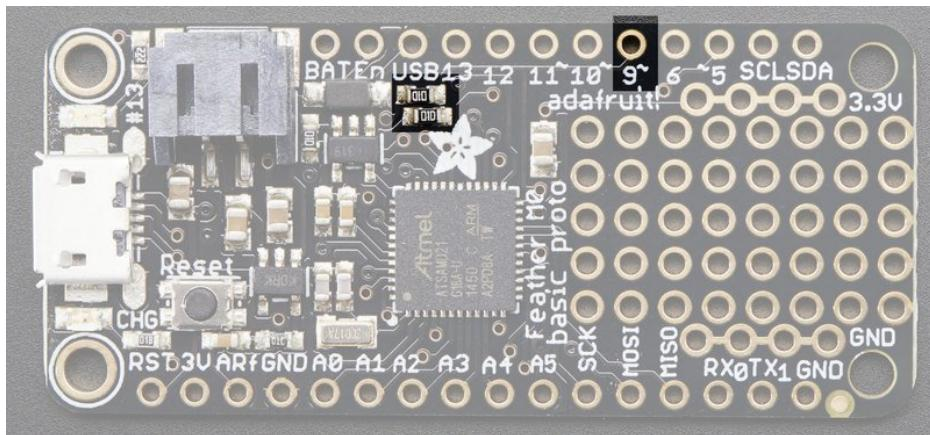
In Arduino, you can read this pin's voltage, then double it, to get the battery voltage.
