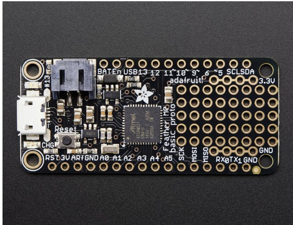
At the Feather M0's heart is an ATSAMD21G18 ARM Cortex M0 processor, clocked at 48 MHz and at 3.3V logic, the same one used in the new [Arduino Zero](http://adafru.it/2843) (<http://adafru.it/2843>). This chip has a whopping 256K of FLASH (8x more than the Atmega328 or 32u4) and 32K of RAM (16x as much)! This chip comes with built in USB so it has USB-to-Serial program & debug capability built in with no need for an FTDI-like chip.
