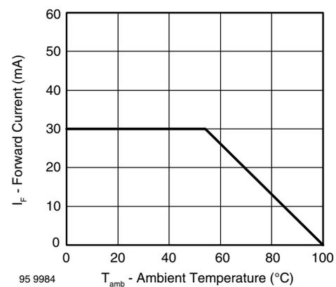
Fig. 2 - Forward Current vs. Ambient Temperature for InGaN
