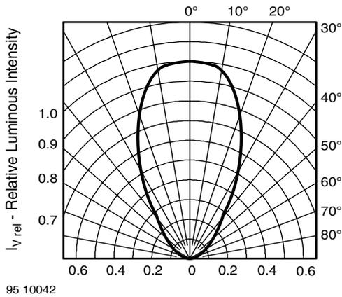
Fig. 4 - Relative Luminous Intensity vs. Angular Displacement
