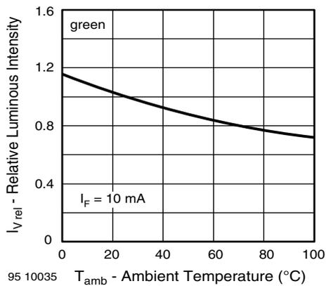
Fig. 11 - Relative Luminous Intensity vs. Ambient Temperature
