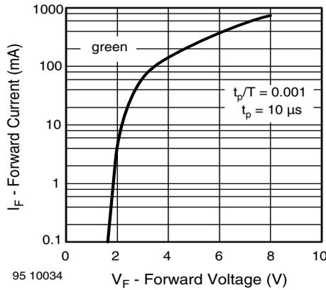
Fig. 10 - Forward Current vs. Forward Voltage
