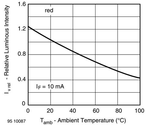
Fig. 6 - Relative Luminous Intensity vs. Ambient Temperature
