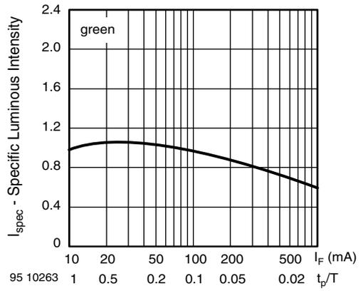
Fig. 12 - Specific Luminous Intensity vs. Forward Current
