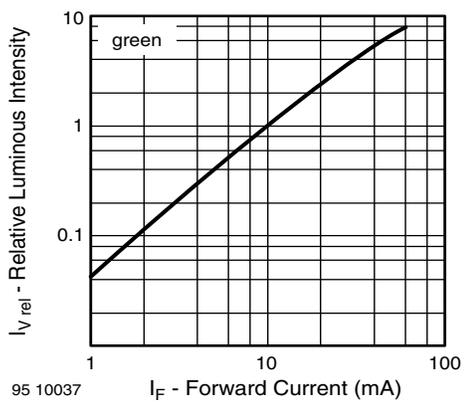
Fig. 13 - Relative Luminous Intensity vs. Forward Current
