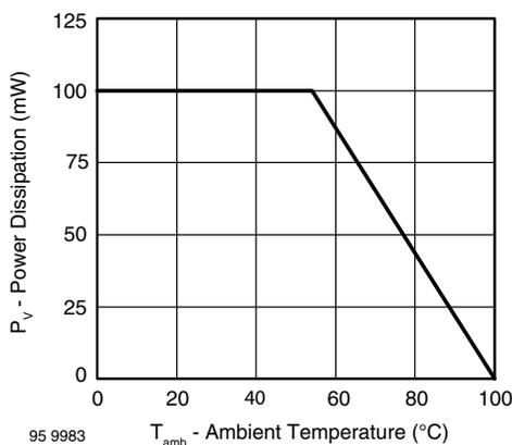
Fig. 1 - Power Dissipation vs. Ambient Temperature
