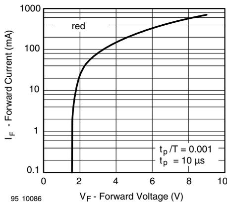
Fig. 5 - Forward Current vs. Forward Voltage
