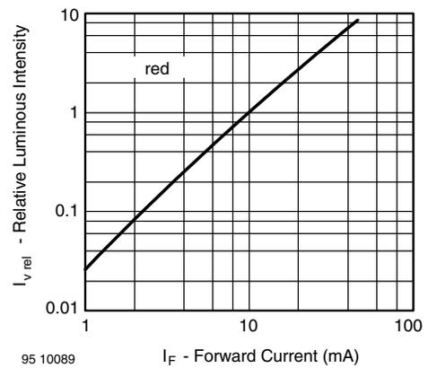
Fig. 8 - Relative Luminous Intensity vs. Forward Current
