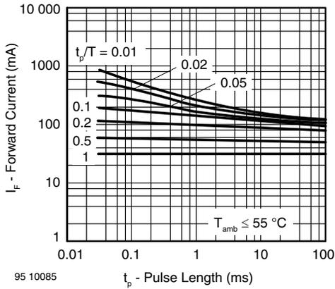
Fig. 3 - Forward Current vs. Pulse Length
